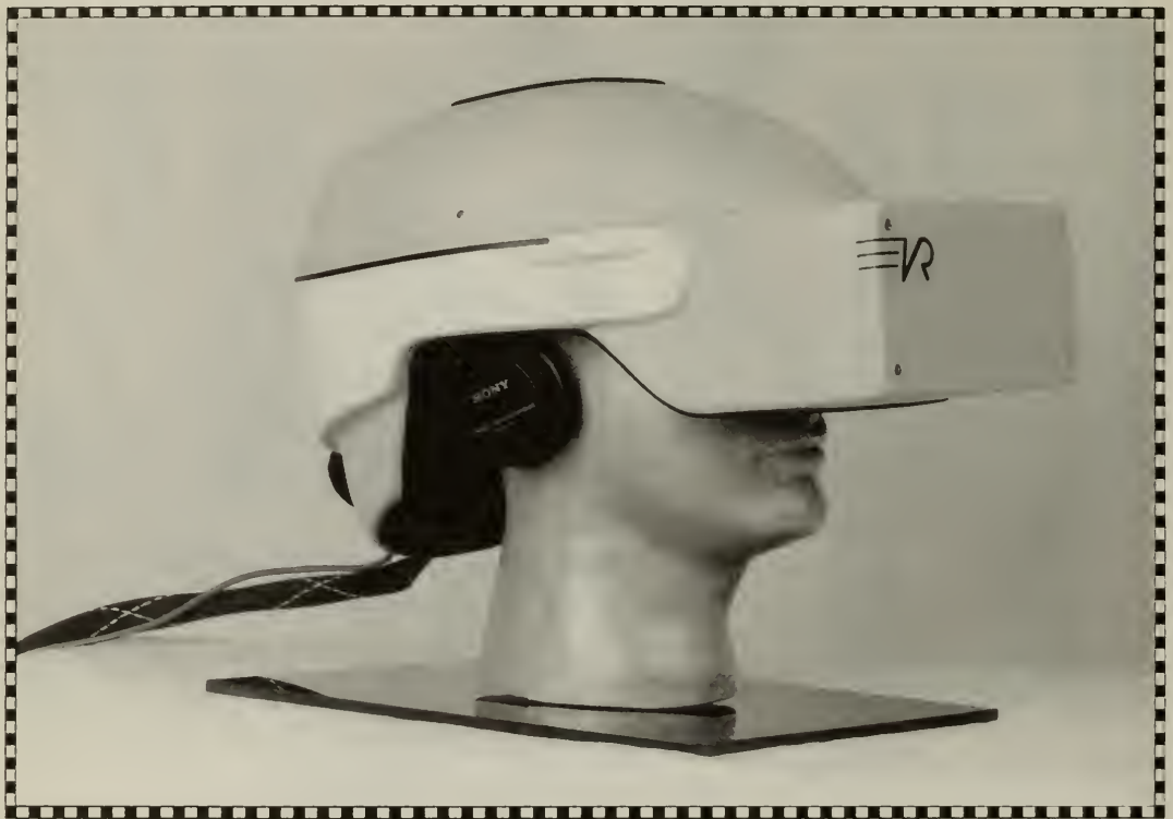
Figure 2.5 This head-mounted display from Virtual Research includes twin displays and built-in stereo headphones
