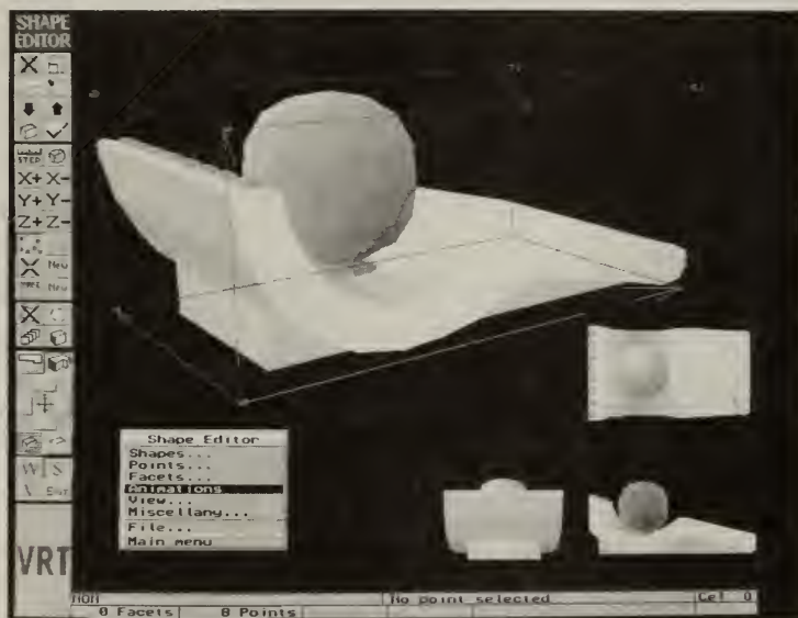
Figure 5.7 The Virtual Reality Toolkit's Shape Editor allows you to design complex, solid, 3D shapes such as a Spaceball controller
