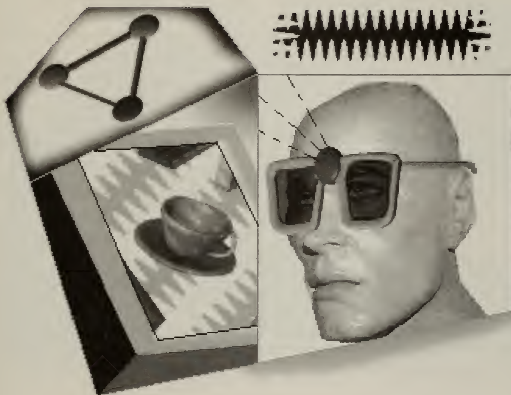
Figure 2.11 The triangular receiver localizes the glasses in three-space to create real-world feedback on the display
