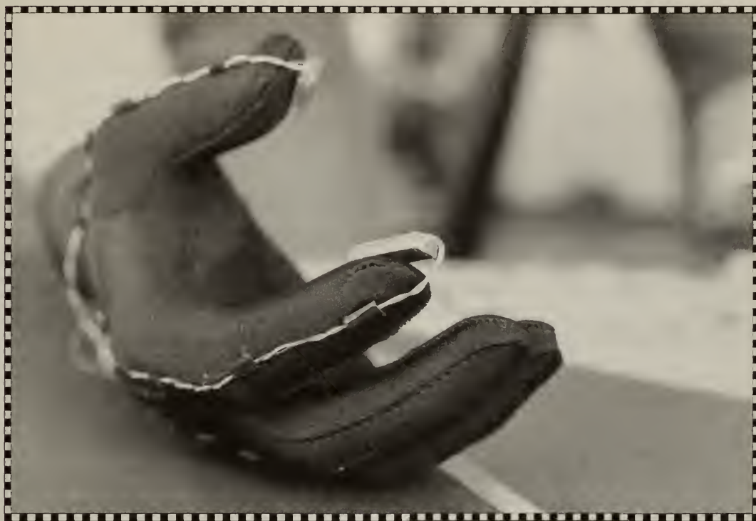
Figure 2.12 Xtenso's tactile feedback gloves let you feel the virtual object you are seeing on the display
