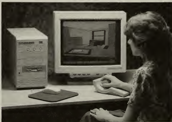
Figure 5.6 Virtual reality hardware distributed by Dimension International includes an enhanced 486 PC and a 6-axis Spaceball controller
