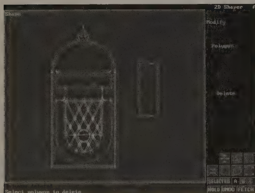
Figure 4-5 The 2D Shaper module is used to create flat shapes from which 3D objects can be constructed
